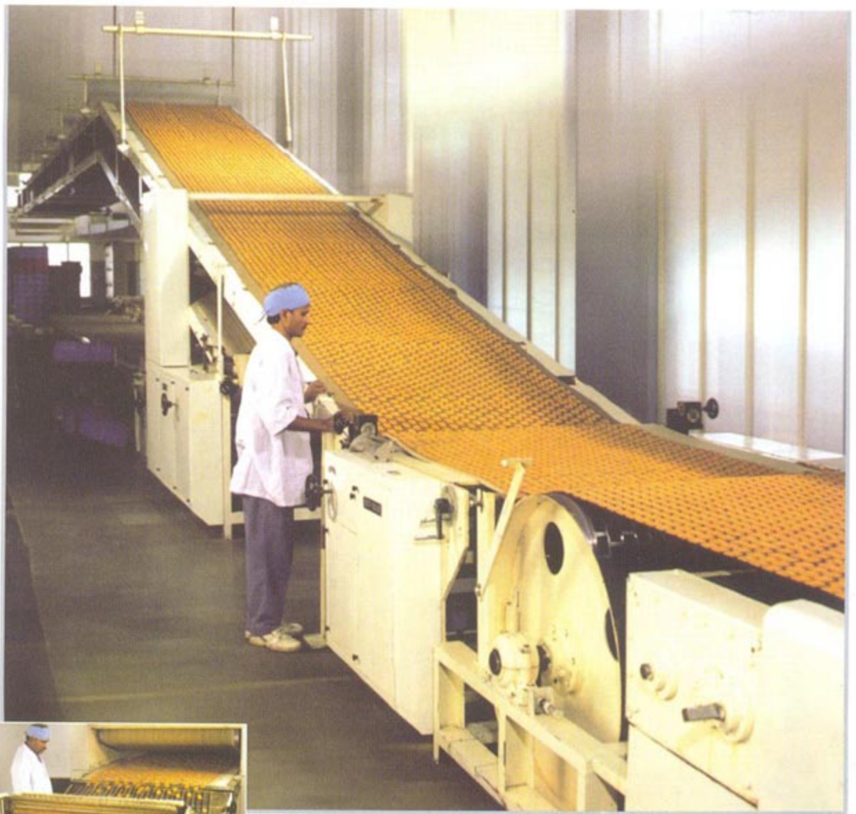
OVERHEAD COOLING CONVEYOR
